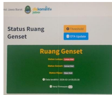
Figure 11. Generator Room Status on the Monitoring Dashboard
