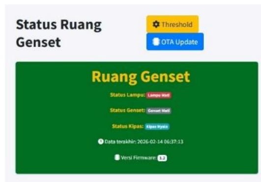
Figure 13. Generator Room Status After the Generator Warm-Up Process
