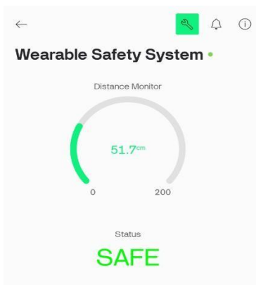
Figure 3. Real-Time Monitoring Interface on the Blynk Application
